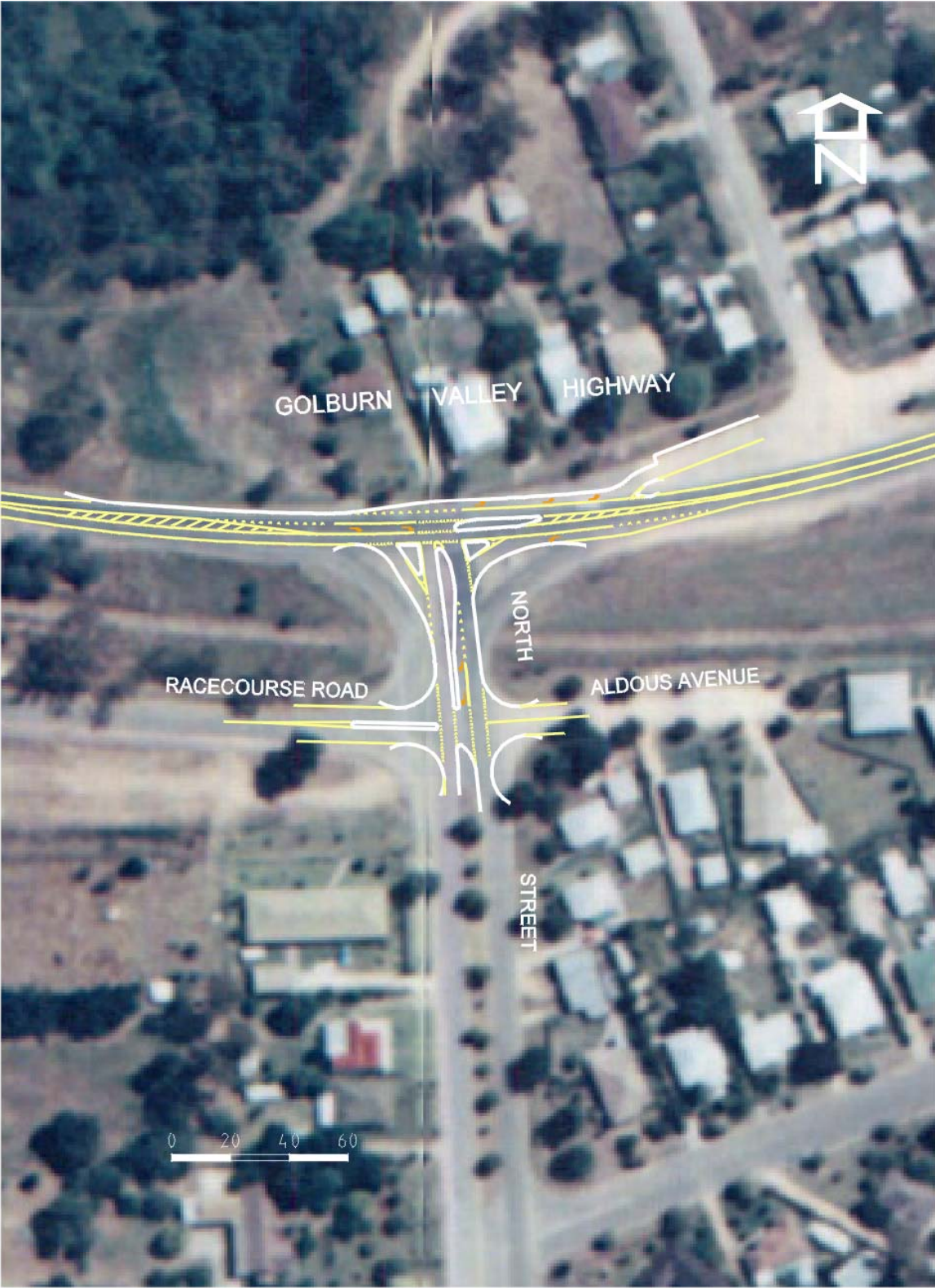
Concept for intersection of North Street at Goulburn Valley Highway, including the adjacent Racecourse Road/Aldous Ave intersection.
